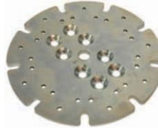
PCD's are great for thick coating removal, very aggressive. For best results remove bulk of coating without continued contact with concrete. Come back with an aggressive metal bond diamond segment and clean up any thin coating left behind. This will help preserve the life of the PCD segments.
